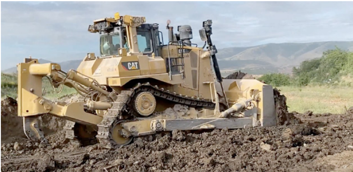
Bulldozers with large ripper tines as illustrated above are commonly used for ripping in the Western Cape.
