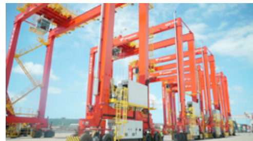
Rubber Tyre Gantry Crane (RTG)
