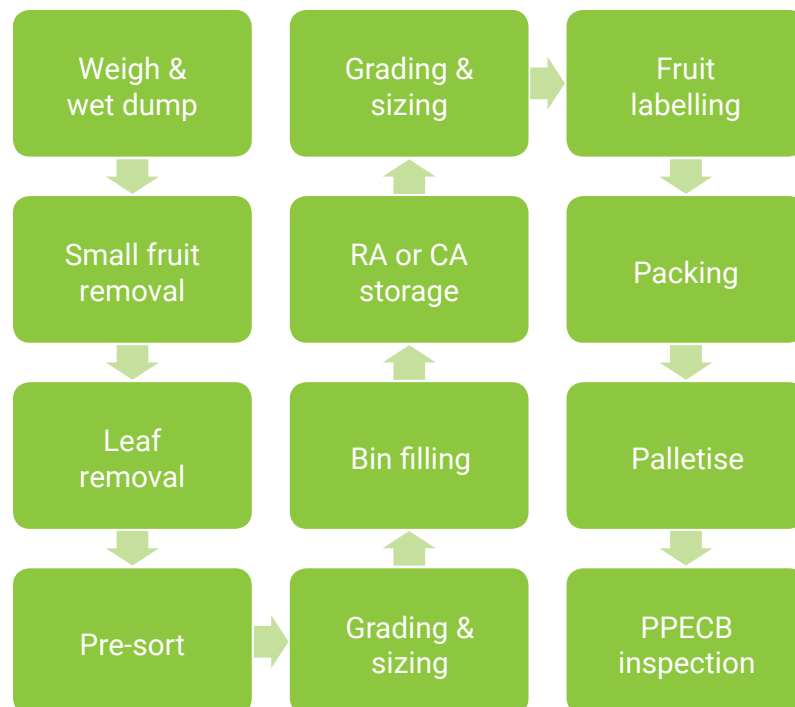
DIAGRAM ILLUSTRATING THE TYPICAL FLOW IN A POME FRUIT PACKHOUSE
